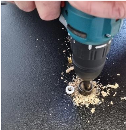
Picture 7: Drilling a hole for couplers
