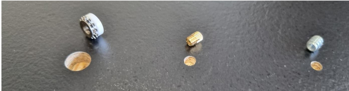
Picture 8: Drilled holes for couplers
