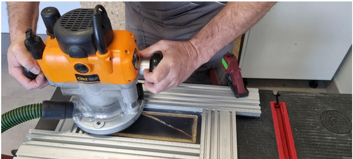
Picture 3: Milling a hole using a plunge cutter and a template
